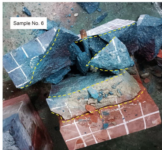
Fig. 8. Fracture morphology of sample No. 6.
