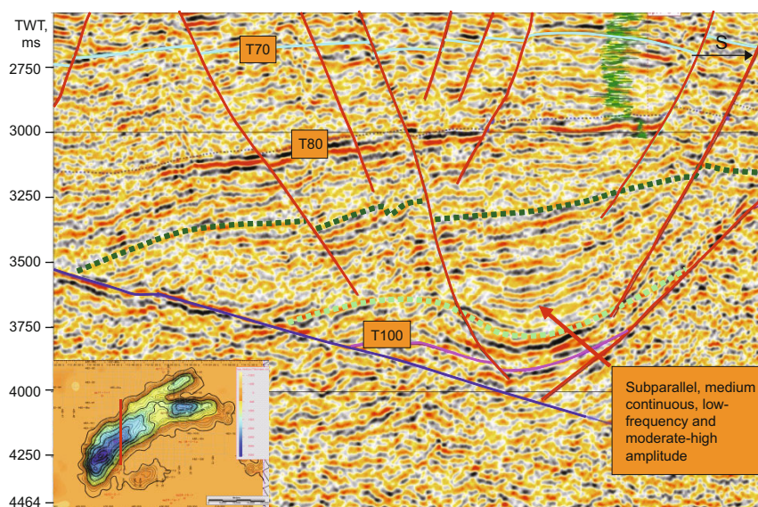
Fig. 5 Seismic reflection characteristics of the Wenchang Formation in the EP17 sub-sag
