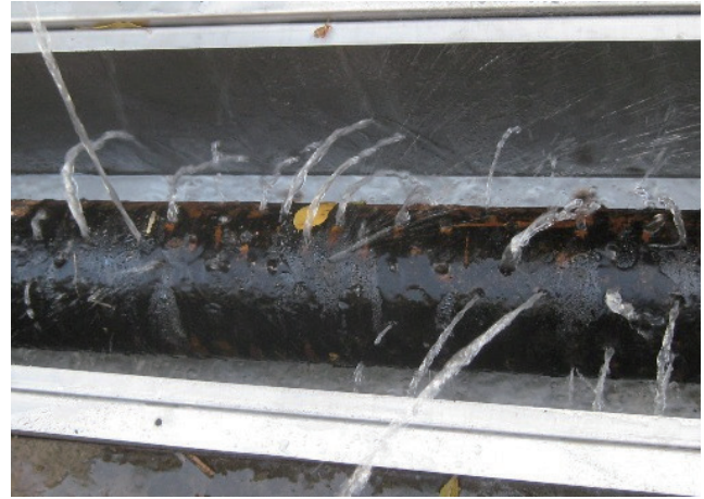
Fig. 5 Photograph of outlet flow at location B of screen No. 1 after cleanup
