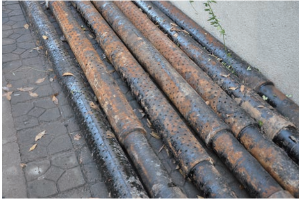
Fig. 3 Plugged metal cotton screens used in the tests
