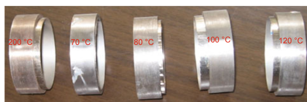
Fig. 7 The appearance of some samples after shearing test
