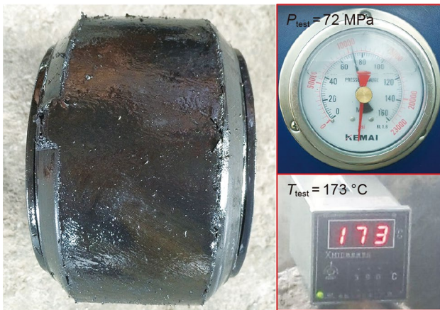
Fig. 20 New packer rubber made of AFLAS with expanding back-up rings after the test
