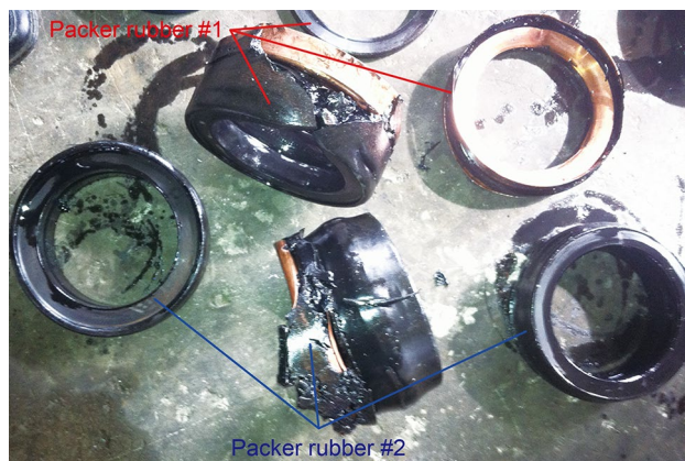
Fig. 13 Ruptured packer rubber made of HNBR
