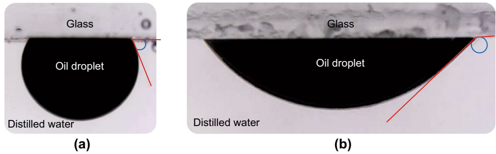
Fig. 6 Close-up views of an oil droplet on the glass surface before (a) and after (b) being aged with stearic acid
