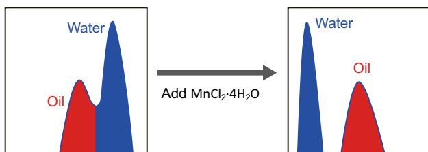
Fig. 11 1D NMR spectrum peak aliasing overlap phenomenon solved by adding chemical reagents in the laboratory
