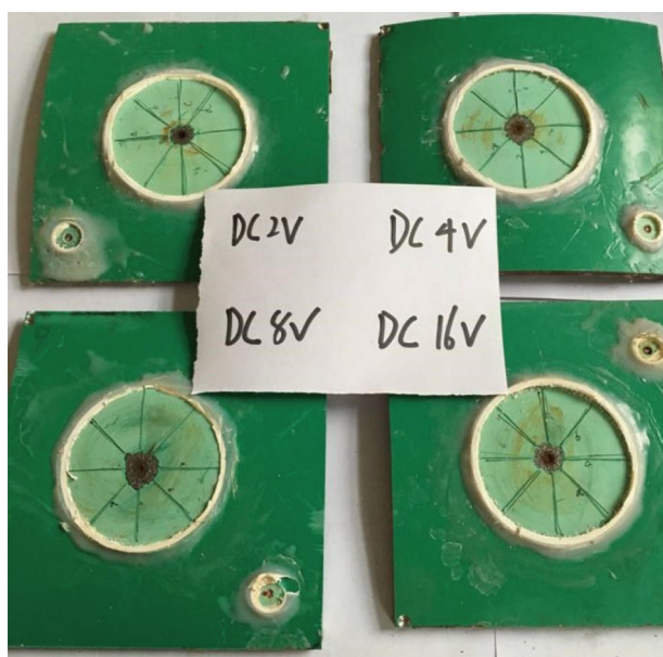
Fig. 10 Cathodic disbonding diagram with positive DC interference
