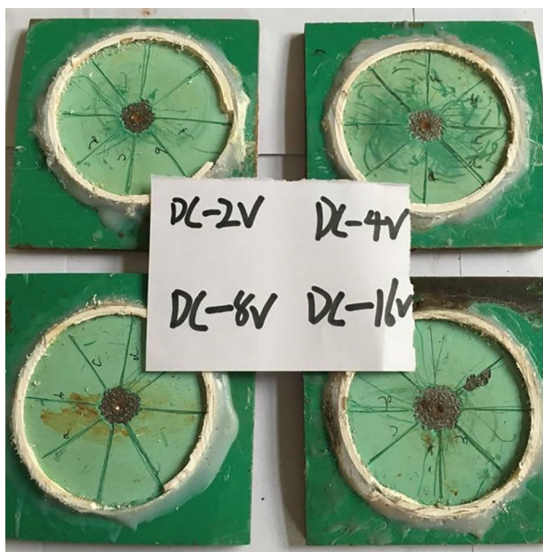
Fig. 15 Cathodic disbonding diagram with negative DC interference
