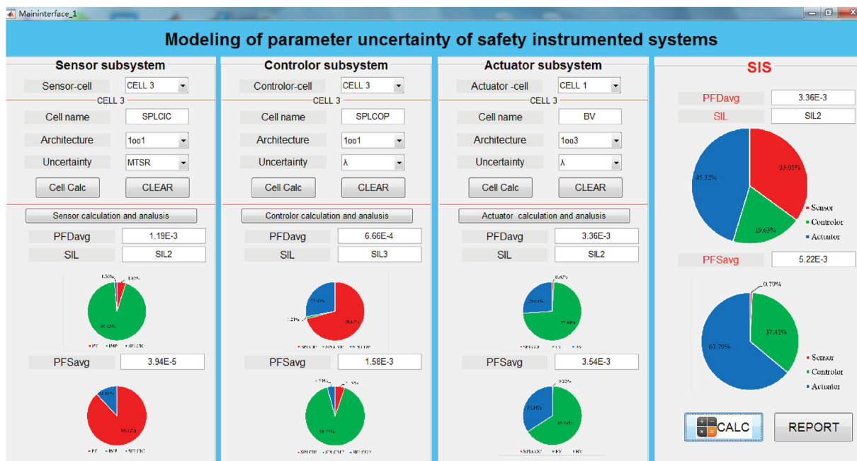
Fig. 18. Main interface of the SIL determination software.
