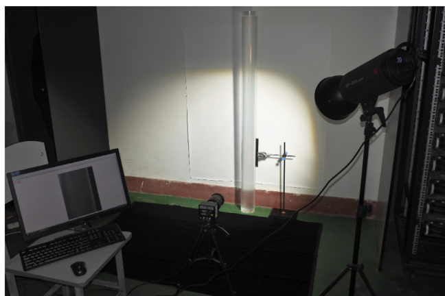
Fig. 1. Experimental setup layout to measure the settling velocity.
