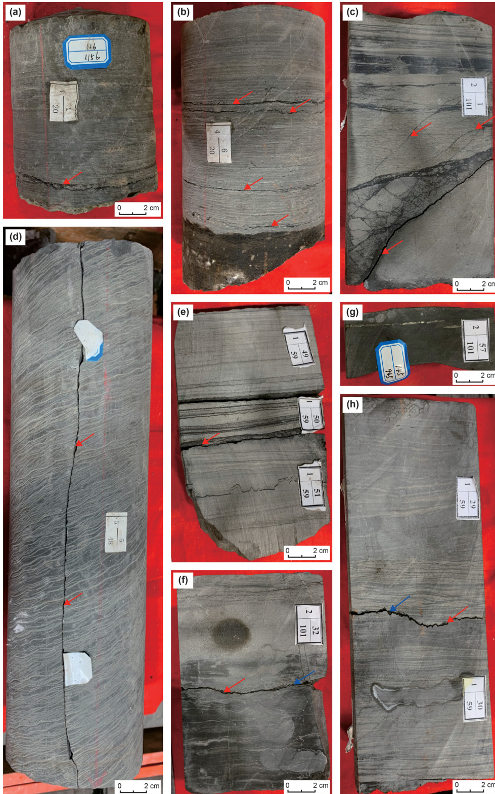
Fig. 2. Core photos show the bedding fractures in Lucaogou Formation, Jimusar Sag. (a). Jagged bedding fractures, J10012, 3293.01m. (b). Three distinct bedding fractures parallel to bedding planes, J10012, 3294.13m. (c). Inclined fractures, J10016. (d). Vertical fractures, J10012. (e). Minerals filling in the bedding planes, J10016. (f). Dissolution and cementation along the bedding surfaces, J10016. (g). Pyrite filling in the bedding planes, J10016. (h). Dissolution and cementation along the bedding surfaces, J10016.
