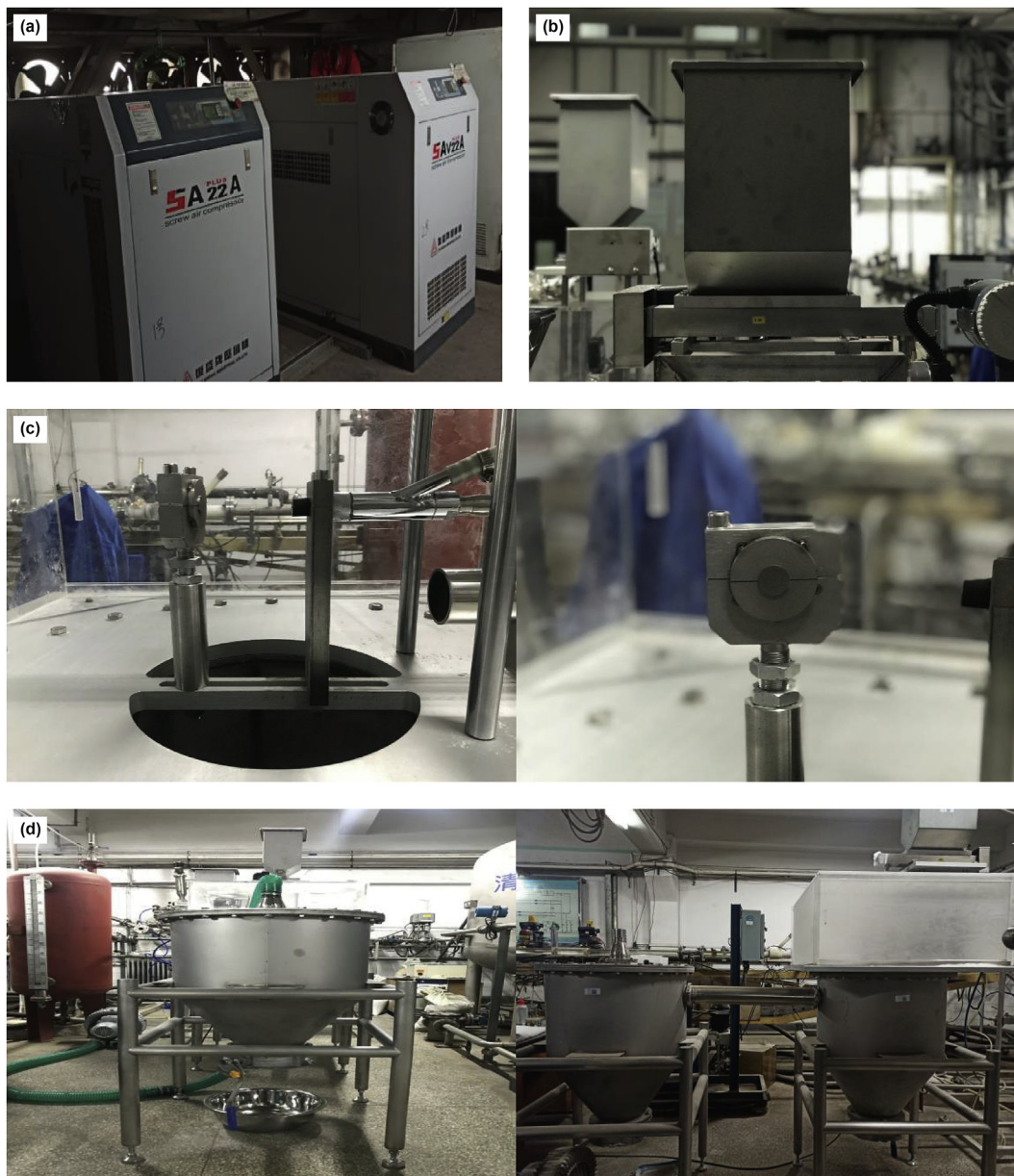
Fig. 2. Gas-solid two-phase erosion device: (a) compression system, (b) feeding system, (c) erosion system and (d) particle recovery system.
