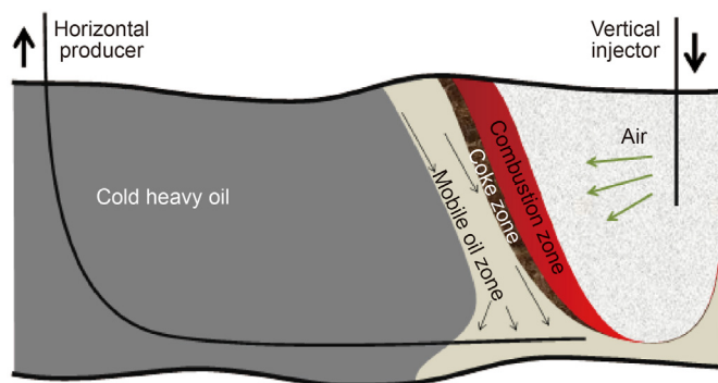
Fig. 1. Schematic of toe-to-heel air injection (THAI) (Greaves and Turta, 1997).
