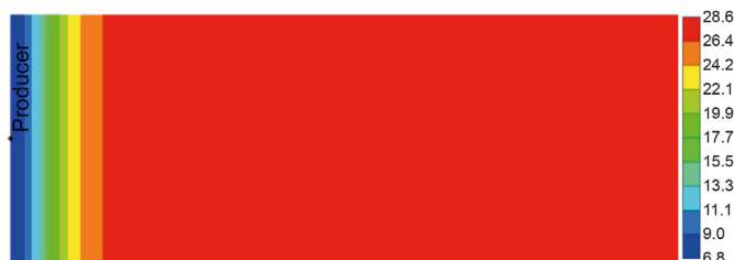
Fig. 3. Gridblock pressures at early time generated using the reservoir simulation model.
