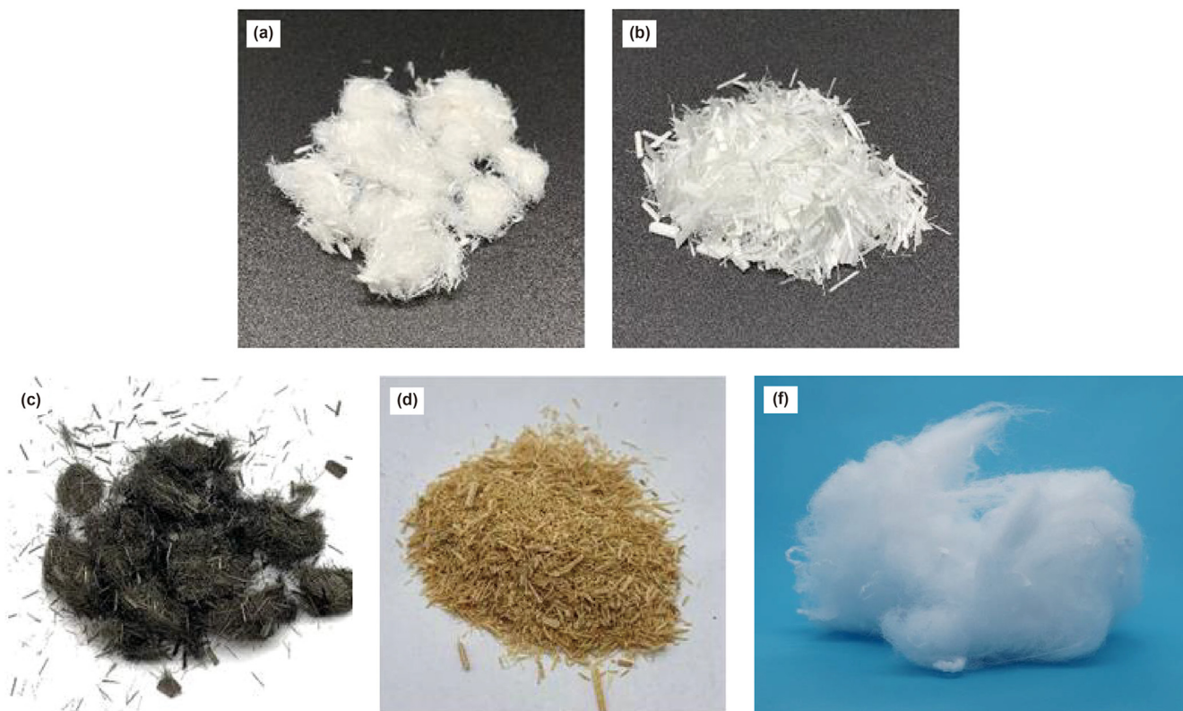
Fig. 13. Images of five different types of fibers used in oil and gas sub-surface stimulations: (a) polyester fiber, (b) polypropylene fiber, (c) carbon fiber, (d) bamboo fiber, and (f) polylactic acid fiber.
