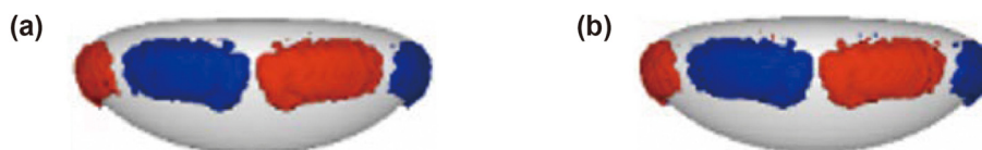
Fig. 12. The streamwise vortices structure of the free bubble at t^* = 25. (a) x - y plane. (b) z - y plane.
