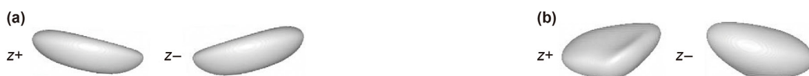
Fig. 17. Comparison of the near-wall bubble shape from two directions of the x - y plane. (a) With a zigzag path. (b) A spiral path.
