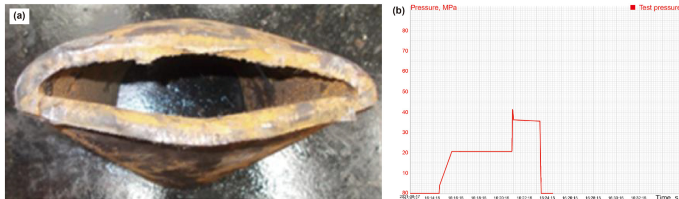
Fig. 13. The final shear result: (a) deformation of the pipe (b) oil pressure curve.
