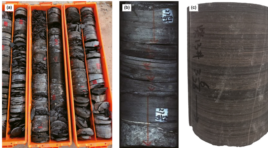
Fig. 1. Unconventional oil and gas reservoir core. (a) Core of Qingshankou Formation, southern Songliao Basin; (b) Core of Longmaxi Formation in Weiyuan, Sichuan Basin; (c) Core of Ganchaigou Formation in Yingxiangling, Qaidam Basin.
