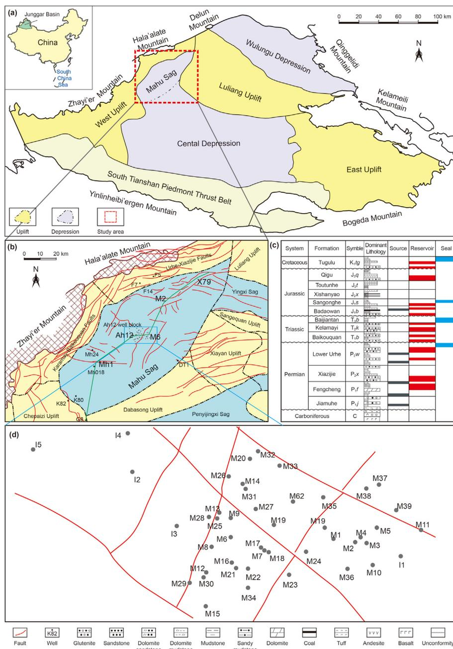
**Fig. 1.** (a) Structural units and location of the study area in the basin; (b) simplified tectonic framework of the Mahu Sag; (c) Comprehensive stratigraphic column of the Mahu Sag, including symbols, dominant lithologies and main petroleum system elements; and (d) location of sampled oil wells in the Ah 12 well block of the Mahu Sag.
