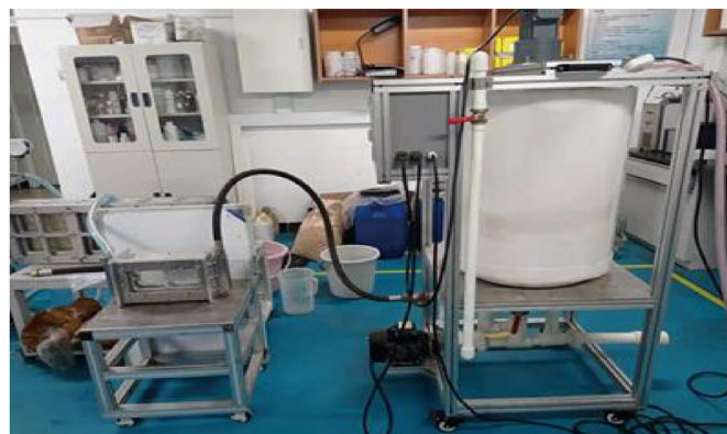
Fig. 4. Experimental system for evaluating temporary plugging performance of high-temperature fractures in hot dry rock.
