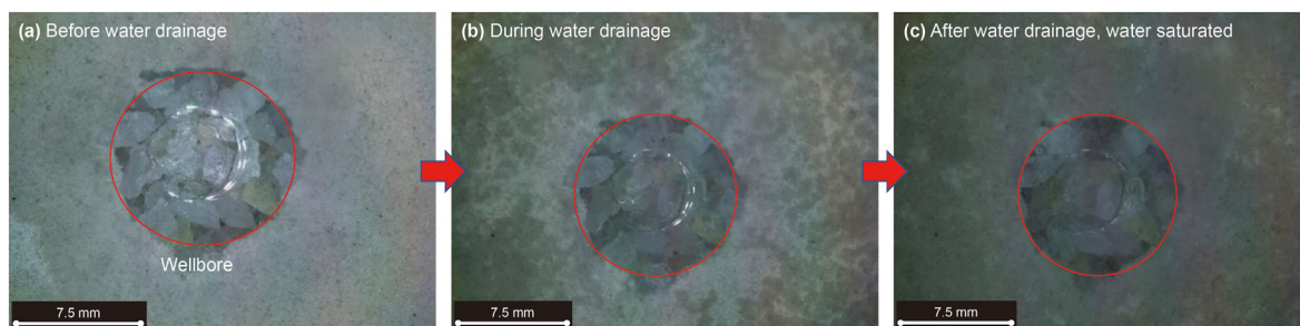
Fig. 5. Optical captures of the simulated wellbore and adjacent HBS before (a), during (b), and after (c) water drainage.
