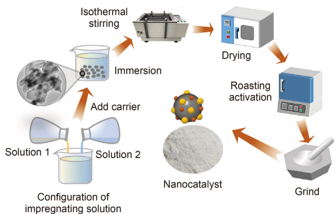
Fig. 1. The preparation process of catalysts.
