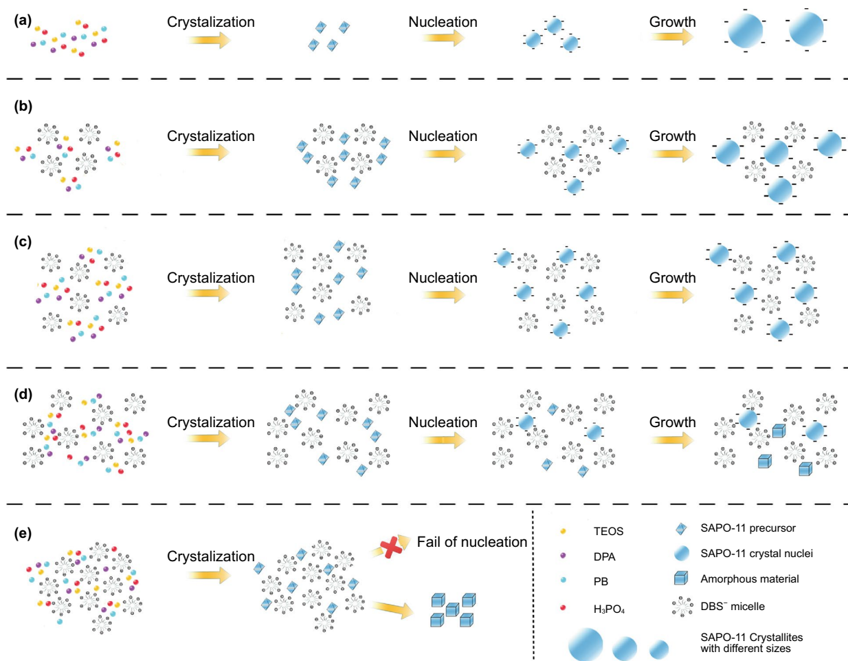
Fig. 3 Schematic diagram of the synthesis principles of S–C (a), S–S 1 and S–S 2 (b), S–S 3 (c), S–S 4 (d) and S–S 5 (e)
