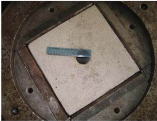
Fig. 11 Cement block with bore hole placed in test cell
