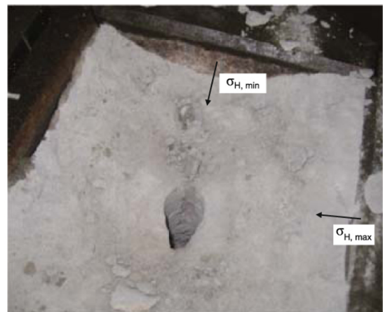
Fig. 14 Collapsed borehole after critical condition
