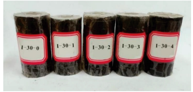
Fig. 1. Propped fracture samples after being dried in a drying oven. Designed fracture widths are 0, 0.8, 1, 2, and 4 mm from left to right.
