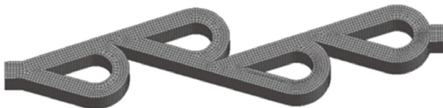
Fig. 5. Fluid region meshing of composite type AICD.
