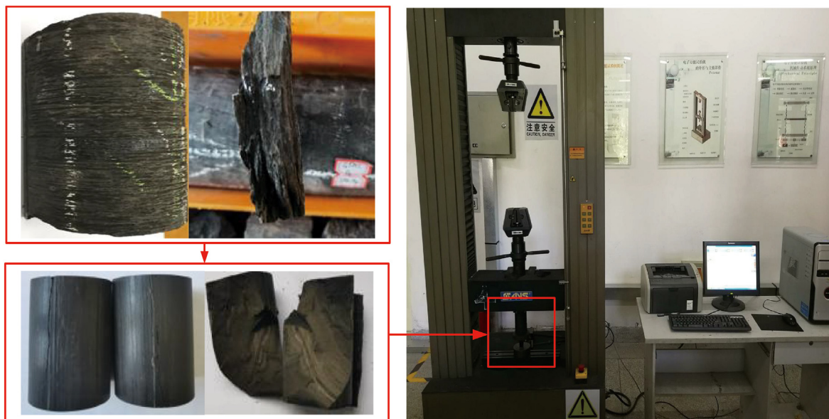
Fig. 7. Uniaxial compression tests of the Gulong shale.
