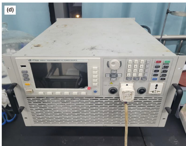
Fig. 2. (a) Microscopic separator for catalyst particle removal; (b) Microscopic experiments; (c) Dry-type power transformer; (d) AC programmable power supply.
