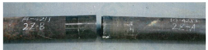
(a) Casing body fracture under tensile load
