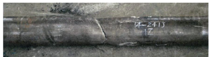
(a) Casing body fracture under tensile load
