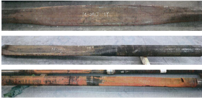
Fig. 18. Casing failure mode under external collapse load.
