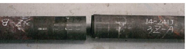
(b) Fracture of the root of external thread under tensile load
