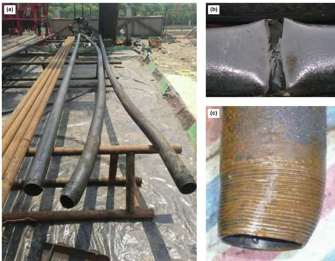
**Fig. 2.** Failure accidents of leaching tubings in the site of salt cavern gas storages, (a) excessive bending, (b) fractured outer tubing, (c) coupling damage (Ge et al., 2021).
