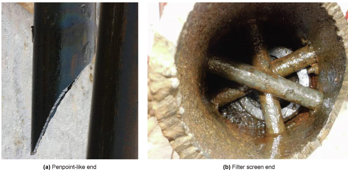
Fig. 8. Two end forms of the inner tubing in engineering site.
