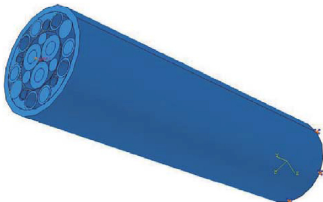
Fig. 3. The FEM model of carbon fiber rod reinforced umbilical cable.
