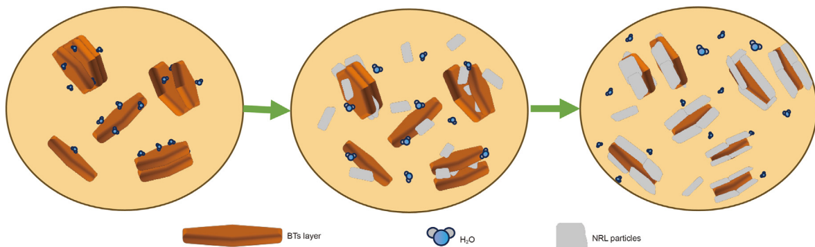
Fig. 9. Schematic illustration of the rheological and filtration control mechanisms of the NRL.
