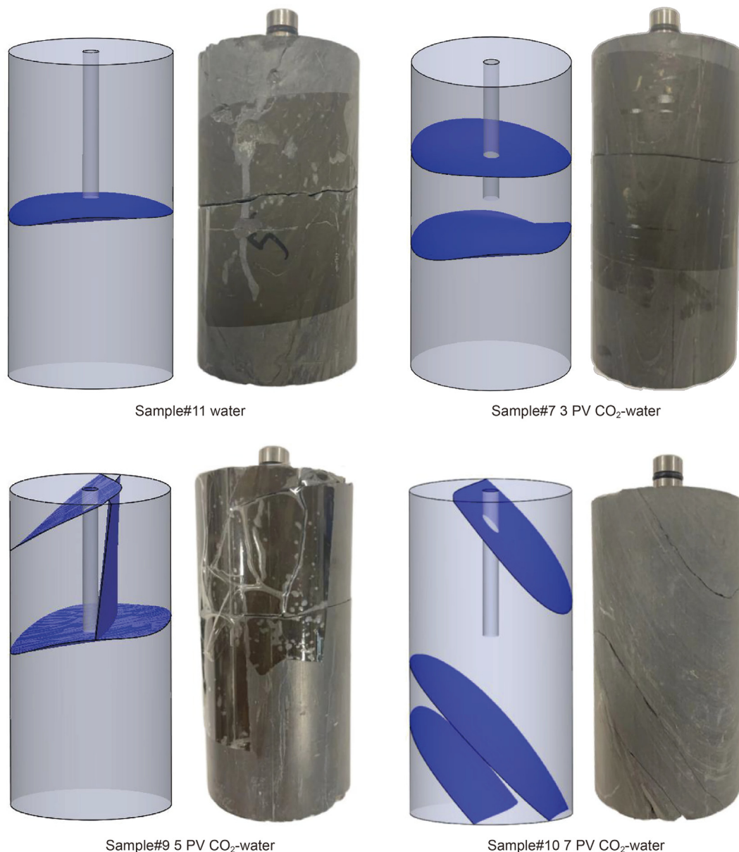
Fig. 8. Schematic diagram of crack reconstruction (water/SC-CO 2 injection volume).
