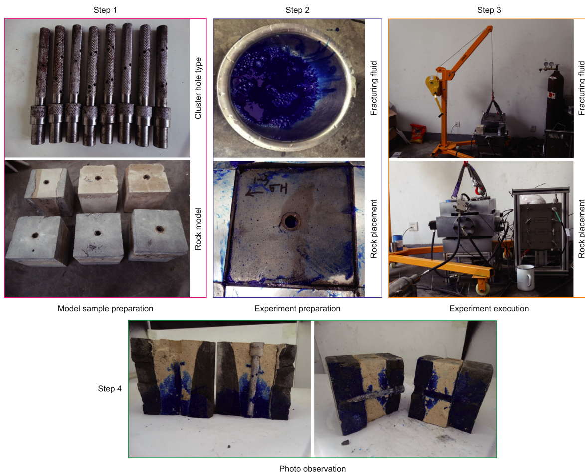
Fig. 2. The experimental configuration and procedure of hydraulic fracturing physical simulation experiment.
