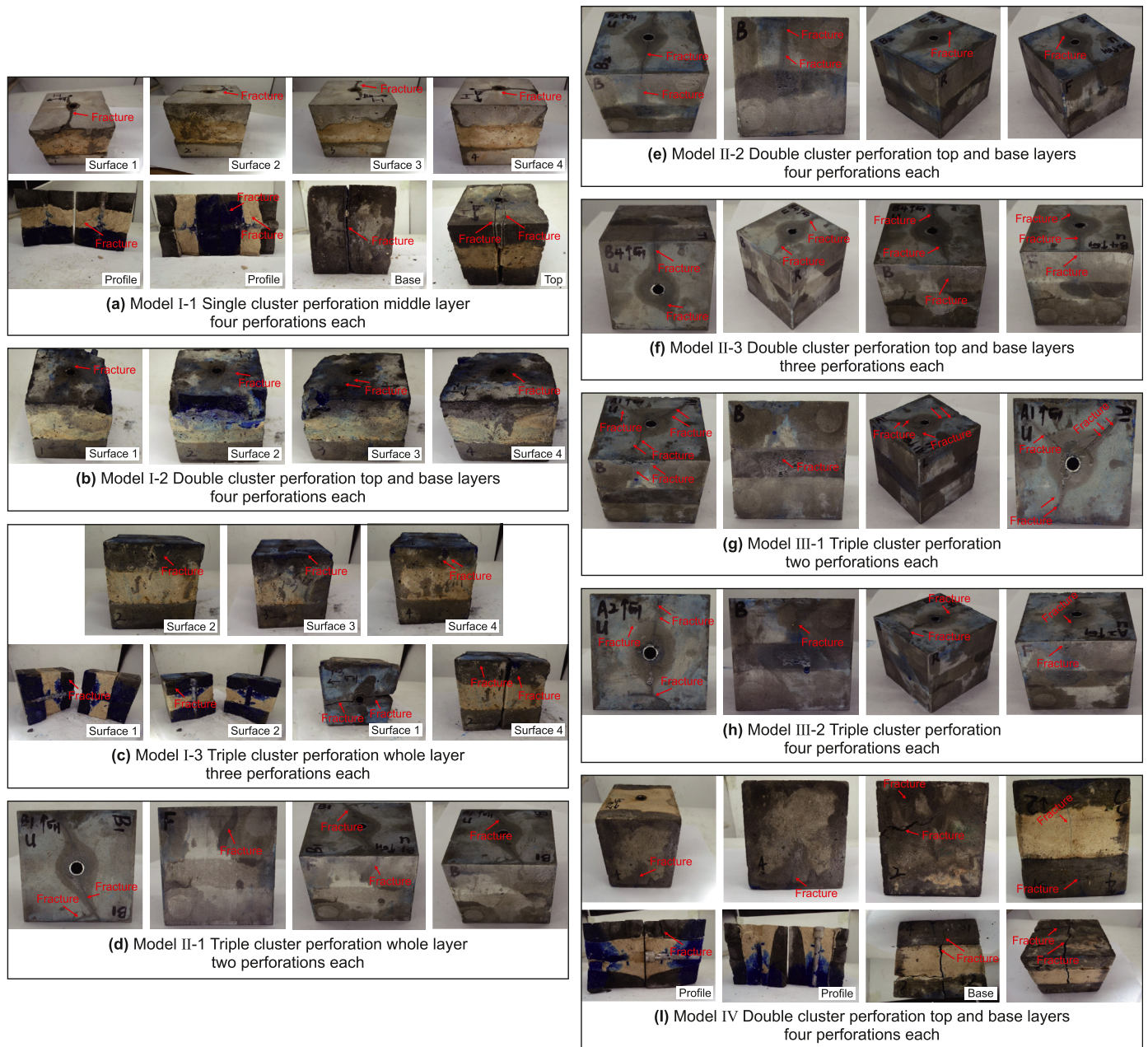
Fig. 8. The results of hydraulic fracturing physical simulation experiment. (a) is the single cluster perforation in middle layer in model I in Fig. 4; (b) refers to the double cluster perforations in top and base layers in model I; (c) shows the triple cluster perforation in whole layer in model I; (d) is the triple cluster perforation in whole layer in model II; (e) refers to the double cluster perforations in top and base layers in model II; (f) indicates the double cluster perforations in model II; (g) is the triple cluster perforation with three perforations each in model III; (h) is the triple cluster perforation with four perforations each in model III; (i) shows the double cluster perforations in top and base layers in model IV. Where surface 1 and 2 are the normal directions of horizontal minimum principal stress; surface 3 and 4 are the normal directions of horizontal maximum principal stress; surface R and L are the normal directions of horizontal minimum principal stress; surface B and F are the normal directions of horizontal maximum principal stress.
