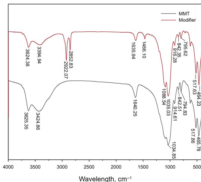
Fig. 4. Infrared spectra of MMT and rheological regulator.
