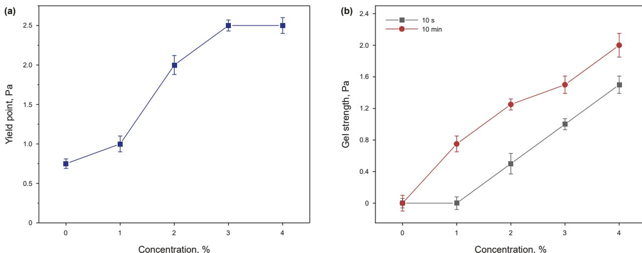
Fig. 11. Variation of yield point and gel strength of drilling fluid with HSCN concentration ((a) yield point; (b) gel strength).
