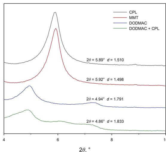
Fig. 5. XRD images of MMT and rheological regulators.
