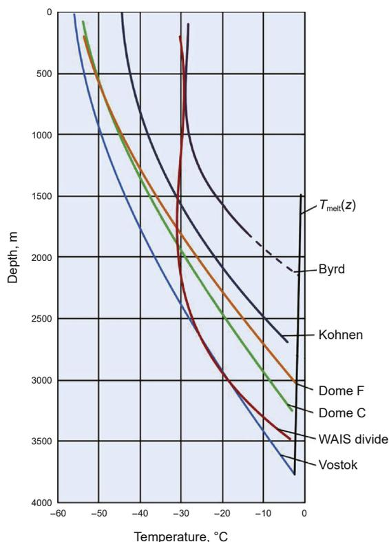
Fig. 1. Variation diagram of ice sheet temperature with depth (Talalay et al., 2020).
