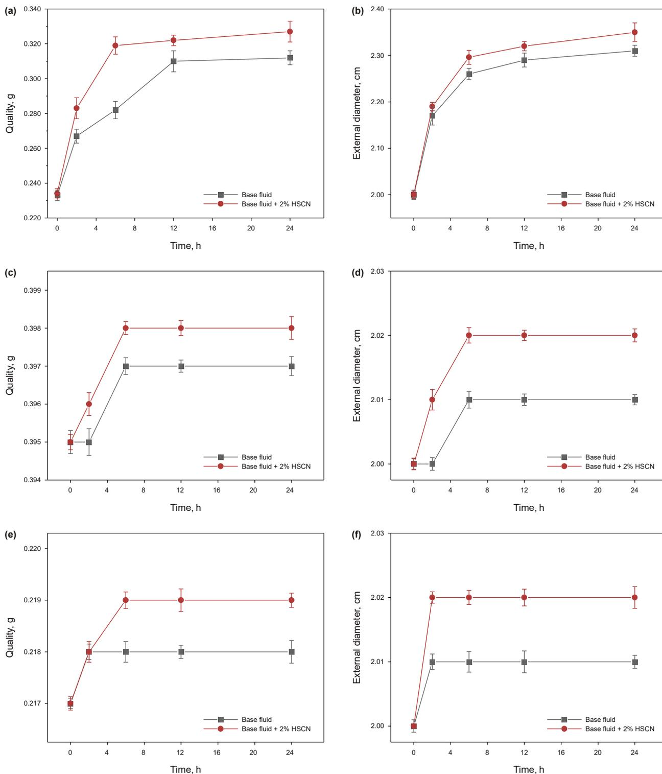
**Fig. 15.** Effect on rubber corrosion ((a) change in mass of silicone rubber; (b) change in outer diameter of silicone rubber; (c) change in mass of fluoroelastomer; (d) change in outer diameter of fluoroelastomer; (e) change in mass of Buna-N; (f) change in outer diameter of Buna-N).
