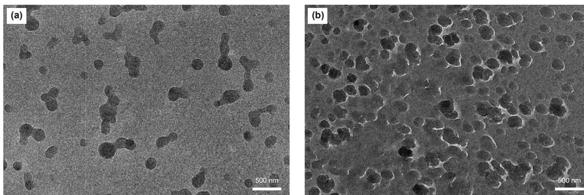
Fig. 19. Images of cryo-transmission electron microscopy ((a) base fluid; (b) base fluid+2% HSCN).
