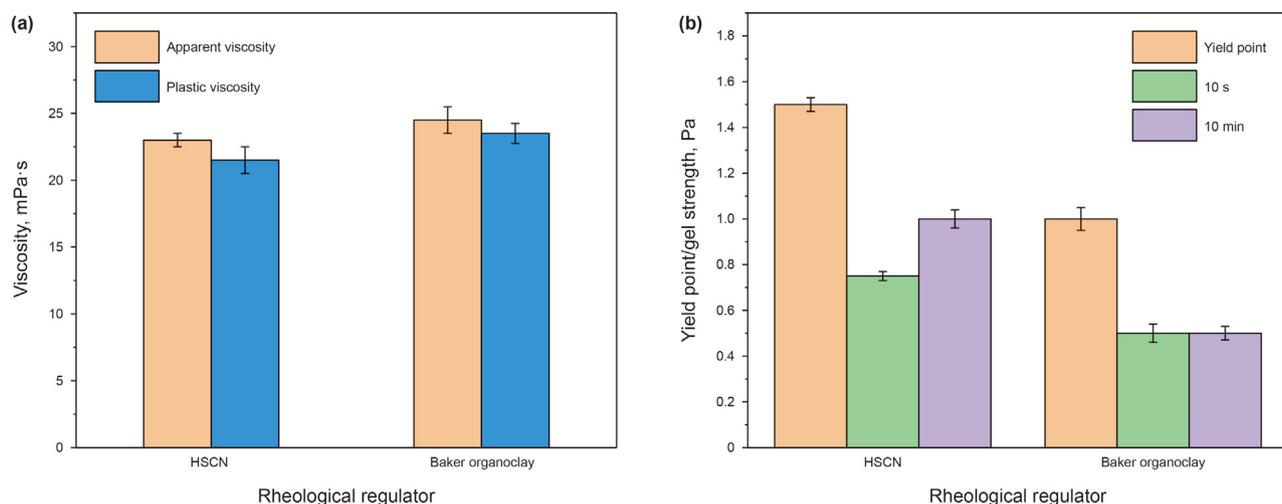
Fig. 12. Comparison of rheological properties between HSCN and Baker organoclay ((a) viscosity; (b) yield point and gel strength).
