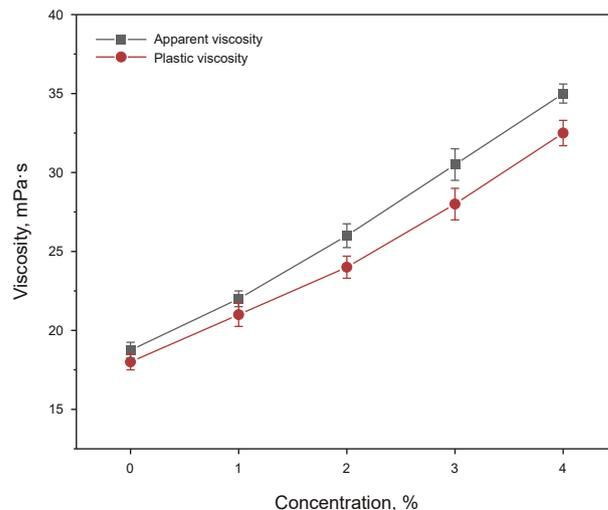
Fig. 10. Variation of drilling fluid viscosity with HSCN concentration.
