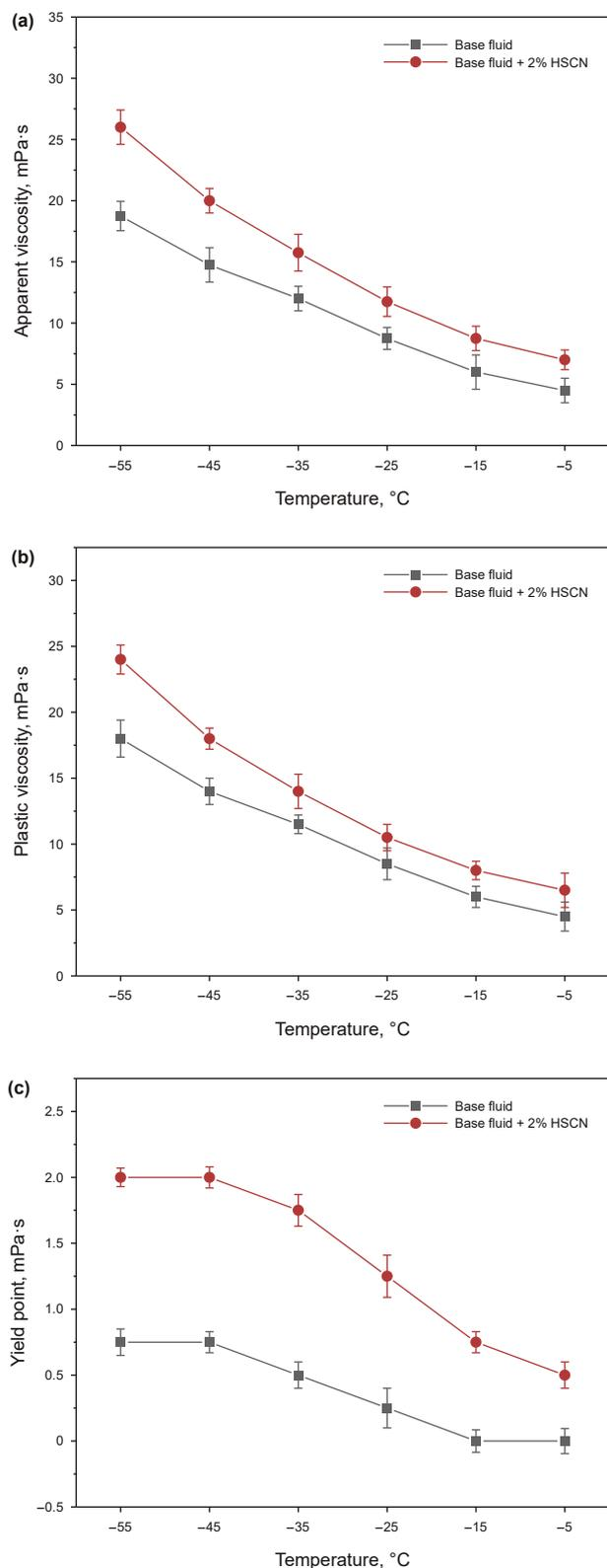
**Fig. 14.** Viscosity-temperature characteristics of drilling fluids ((a) Variation of apparent viscosity with temperature; (b) Variation of plastic viscosity with temperature; (c) Variation of yield point with temperature).
