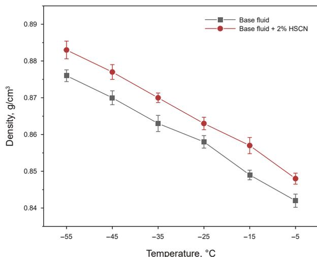
Fig. 16. Variation relationship of drilling fluid density with temperature.
