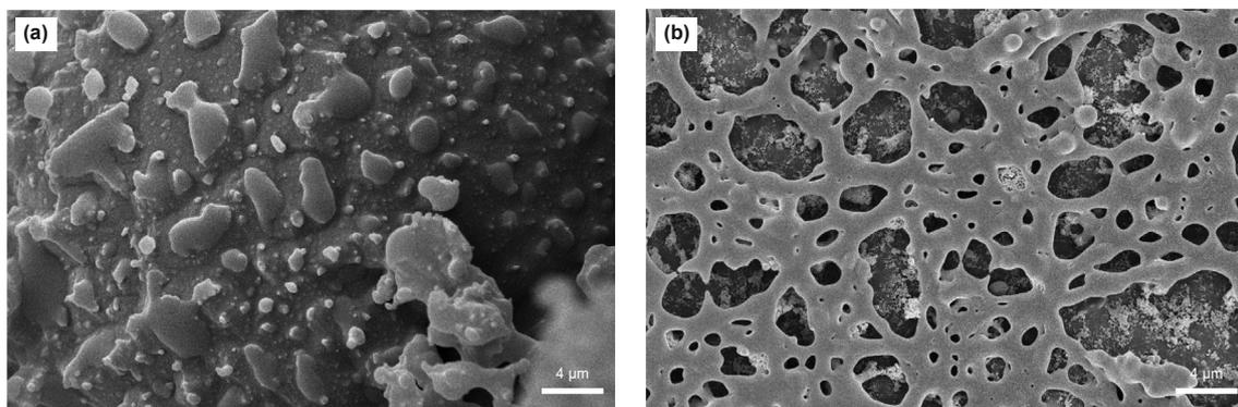
Fig. 18. Images of cryo-scanning electron microscopy ((a) base fluid; (b) base fluid +2% HSCN).
