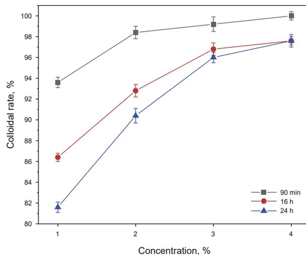
Fig. 9. Variation of colloid rate with HSCN concentration.
