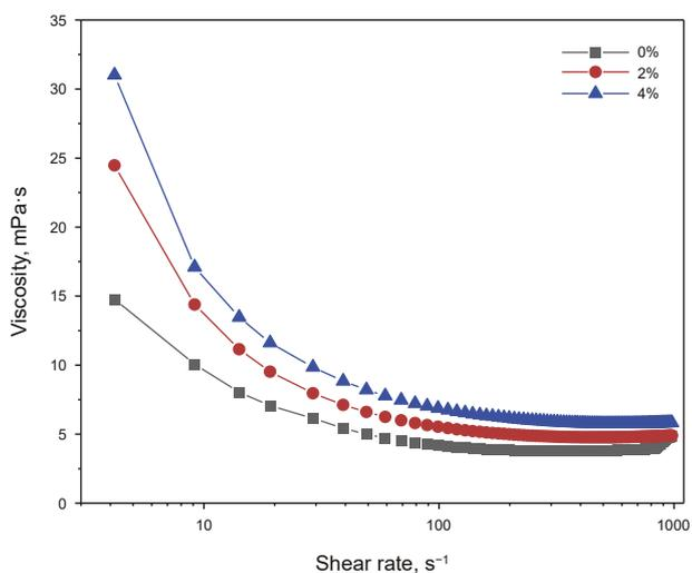
Fig. 13. Variation of drilling fluid viscosity with shear rate.
