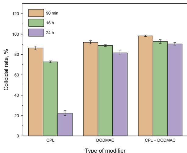
Fig. 8. Effect of different modifiers on the colloidal rate of rheological regulators ((a) CPL-MMT; (b) DODMAC-MMT; (c) (CPL + DODMAC)-MMT).
