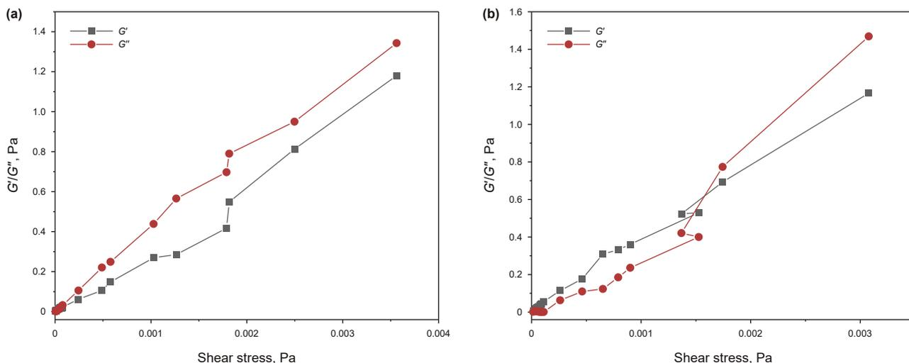
Fig. 17. Variation of drilling fluid modulus with shear stress ((a) base fluid; (b) base fluid +2% HSCN).
