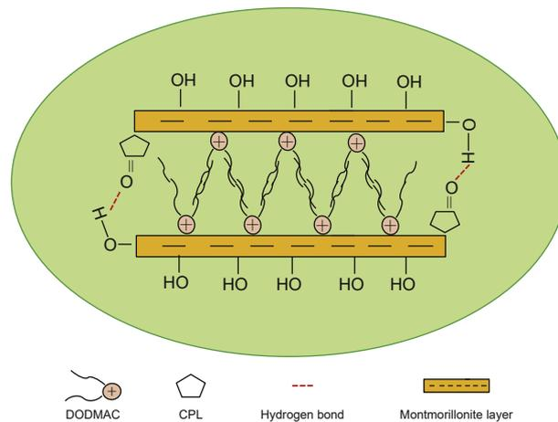
Fig. 3. Structure diagram of rheological regulator (HSCN).
