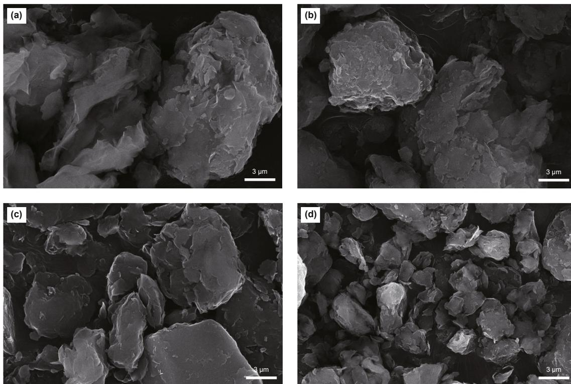
Fig. 6. SEM images of MMT and rheological regulators ((a) MMT; (b) CPL-MMT; (c) DODMAC-MMT; (d) (CPL + DODMAC)-MMT).
