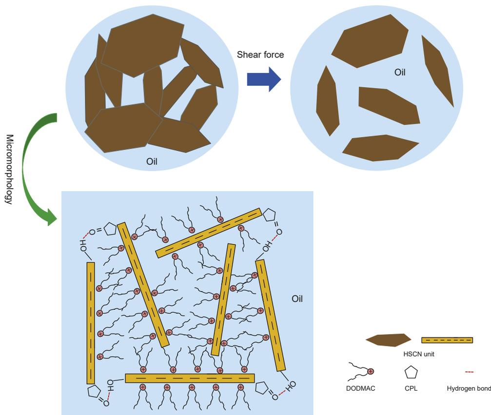
Fig. 20. Schematic diagram of the mechanism of HSCN to improve rheological properties.
