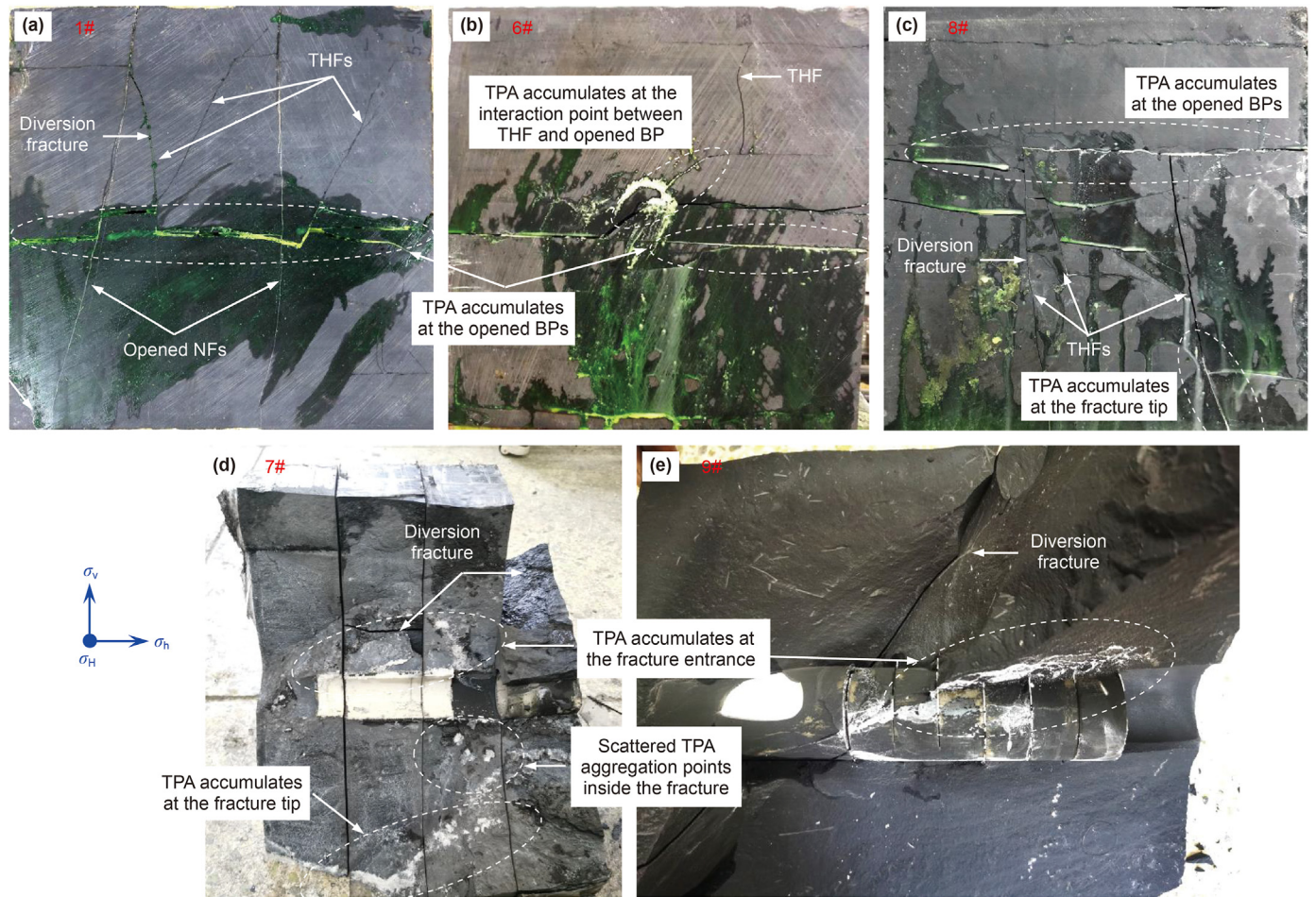
Fig. 8. Distribution of TPA on the surfaces and the interior of five representative specimens. (a) 6#; (b) 8#; (c) 1#; (d) 7 #; (e) 9#.
