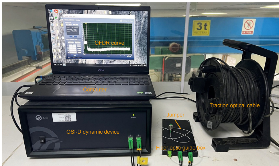
Fig. 1. Photo of optical fiber OSI-D dynamic equipment.
