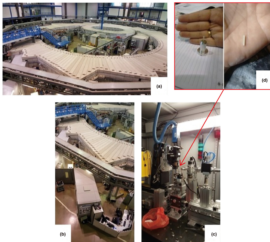
Fig. 6. Schematic summary of the acquiring X-ray computed tomography data. Internal view of the Brazilian Synchrotron Light Laboratory (a), X-ray imaging beamline (b), PCO-2000 white beam microscope (c), and highlighting the sample size (d).
