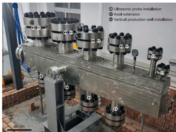
Fig. 4. The fan column-shaped hydrate simulator.
