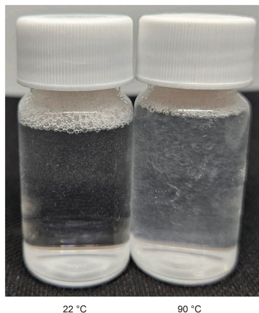
Fig. 4. DTAB solutions (1.00 wt%) in 1 \times \text{HSW} at 22 and 90 °C after 1 week.
