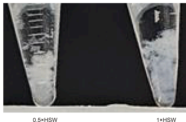
Fig. 2. Precipitation when 1.00 wt% EDTA at high pH value ( \text{pH} = 10.3 ) was added to different brines.
