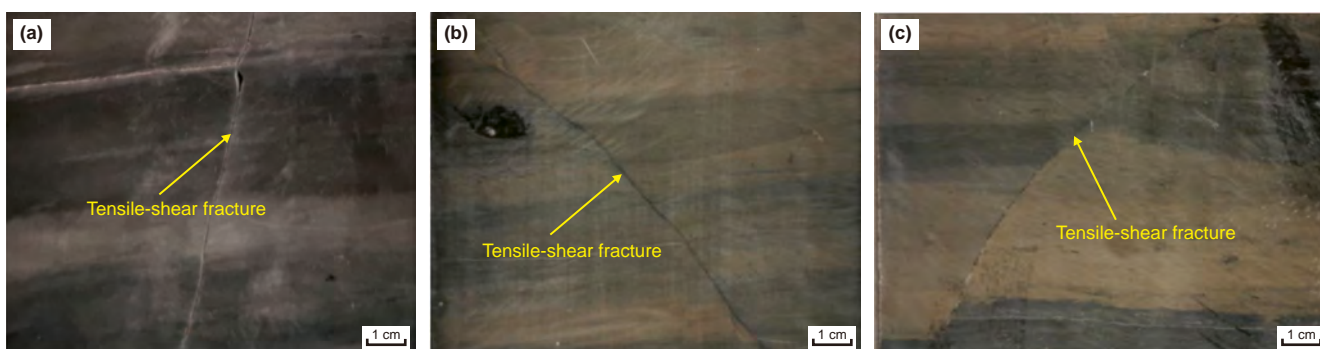
Fig. 3. Core characteristics of tensional-shear fractures. (a) Tensile-shear fracture, form straight, Well GD12, 2976.25 m; (b) tensile-shear fracture, high angle, Well GD12, 2987.65 m; (c) tensile-shear fracture, extend further, Well GD12, 2956.78 m.
