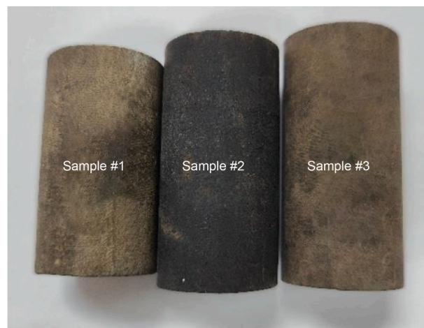
Fig. 1. Experimental core samples from Jimusar shale oil reservoir.
