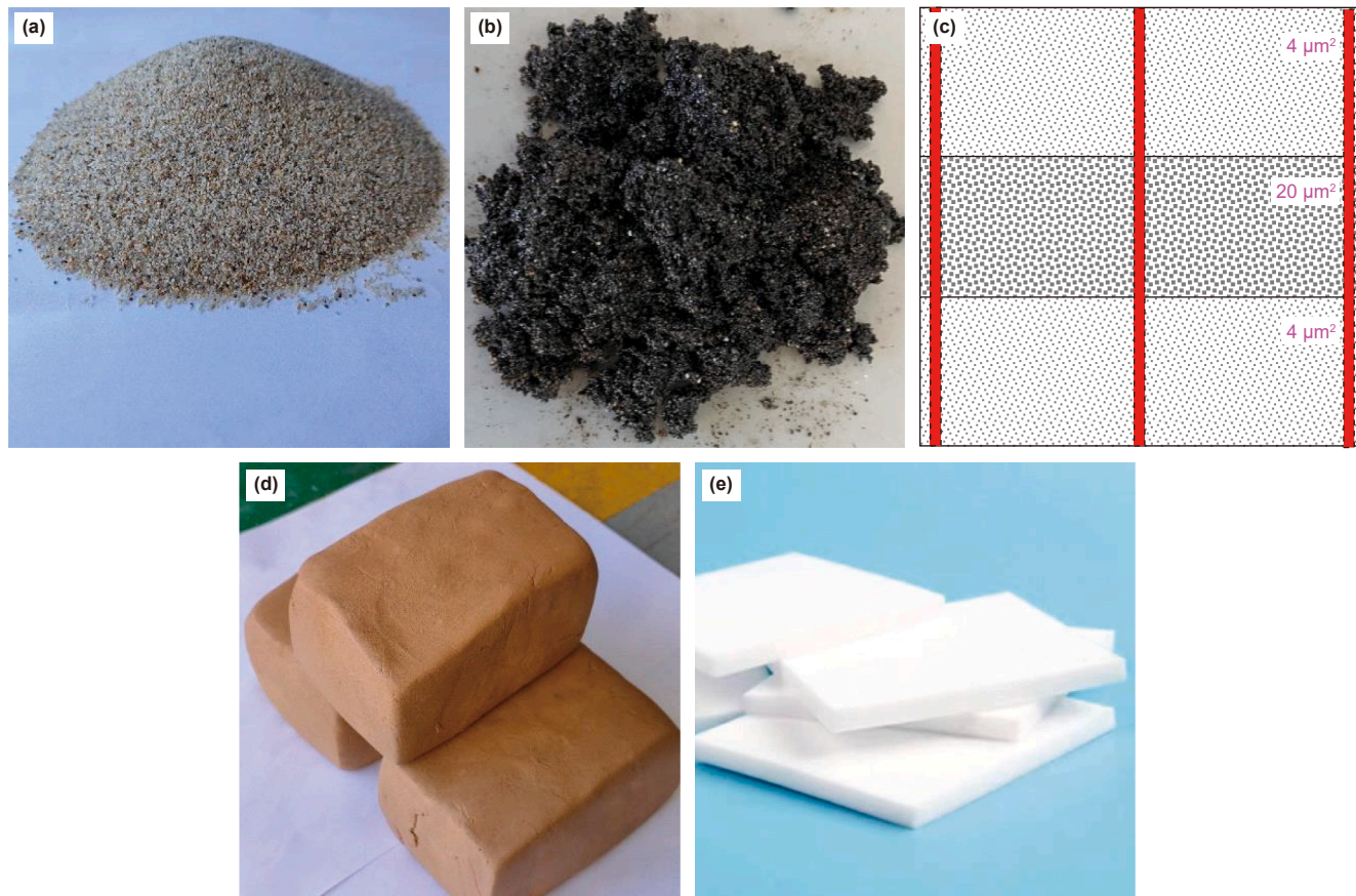
Fig. 5. Materials used in the experiment. (a) Quartz sand; (b) experimental oil sand; (c) oil sand filling method; (d) clay; (e) PTFE sheets.
