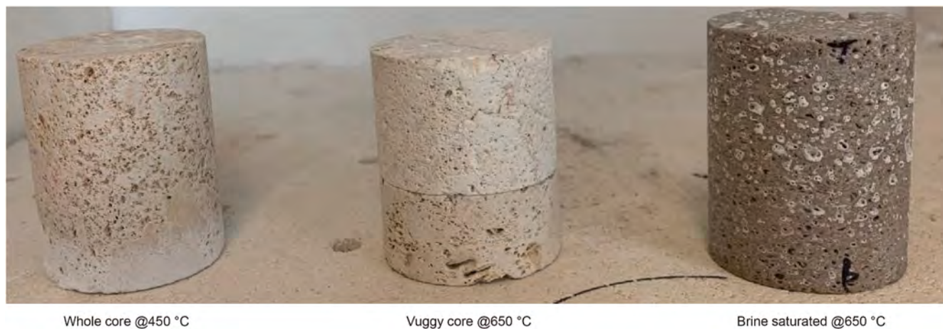
Fig. 20. Photographs of Whole, Vuggy, and Brine saturated cores.
