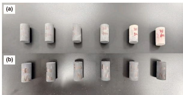
Fig. 1. Two groups of organic-rich shale samples cracking at air (a) and N_2 (b) conditions.
