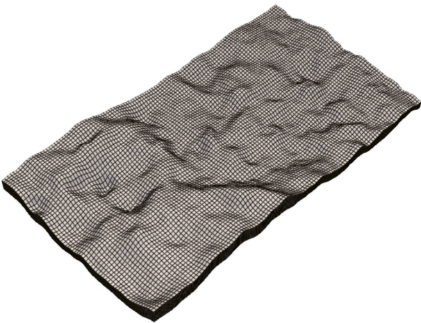
Fig. 14. Reservoir grid of Utsira L7.
