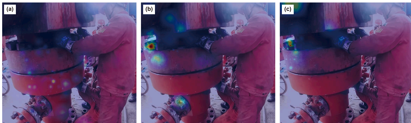
Fig. 7. Comparison of attention visualizations for three different downsampling methods. (a) Avgpooling. (b) Maxpooling. (c) Conv. Among them, avgpooling shows more dispersed attention, effectively attending to various targets; Maxpooling exhibits concentrated and prominent attention; Conv has larger attention errors and poorer performance.
