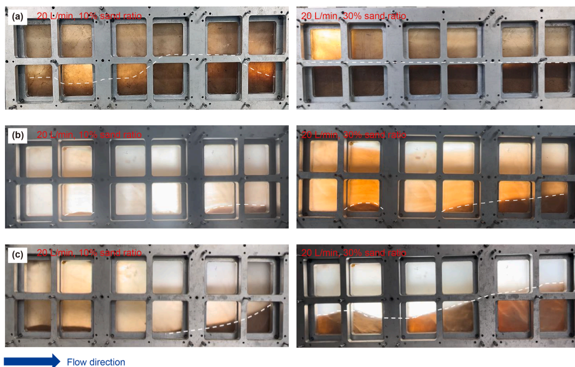
Fig. 9. Comparison of dynamic sand-carrying before and after CRS-10 assembly (different sand ratios). (a) Before the assembly of CRS-10 system; (b) after the assembly of CRS-10 system; (c) field-standard fracturing fluids.
