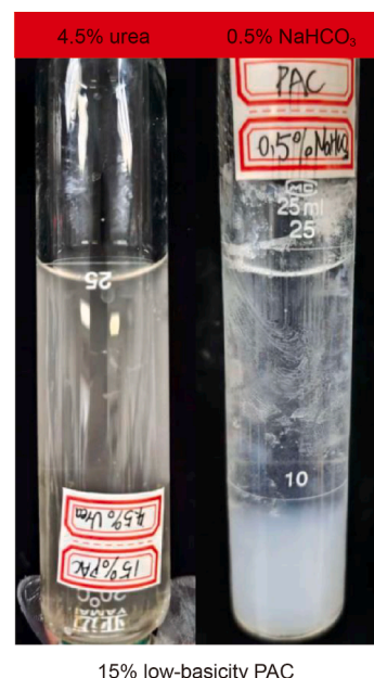
Fig. 4. Gelation behavior of PAC/urea and PAC/NaHCO 3 mixtures.
