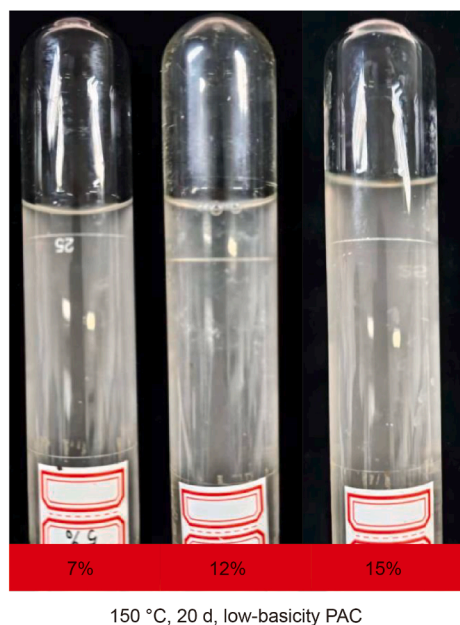
Fig. 3. Gelant appearance of low-basidity PAC at 150 °C.
