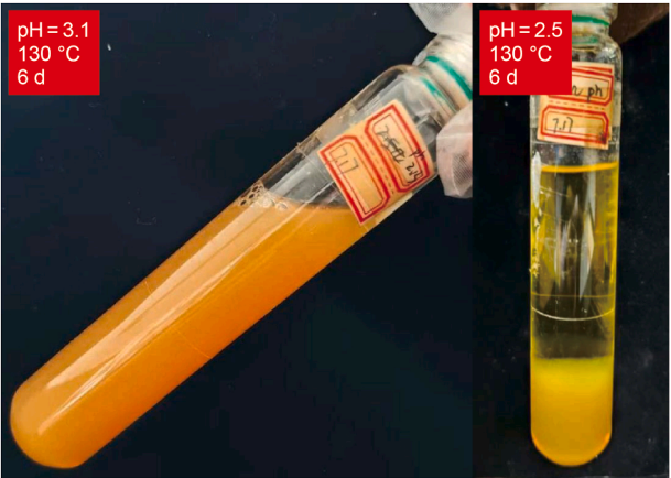
Fig. 7. Effect of pH on the gelation behavior of 12% PAC at 130 °C.
