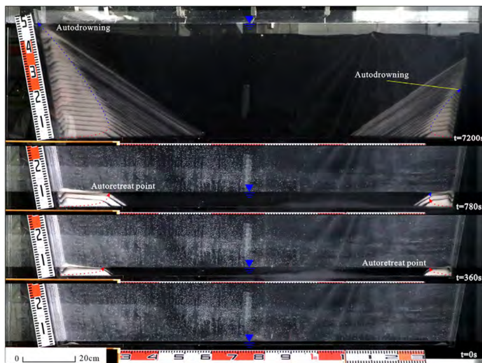
FIGURE 6 | Sequential images recorded in run F-1. Note that transgression in the left provenance occurred at 780s, while in the right provenance, it occurred at 360s.
